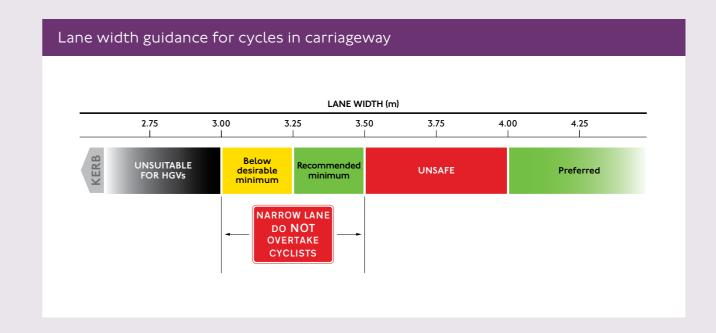
Widths between 3.25 metres and 3.5 metres will allow buses and HGVs to use the lane but it will not be possible for them to overtake cycles.
