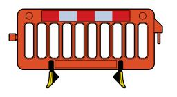
Pedestrian barrier with low-profile feet can reduce obstructive widths and tripping hazards
