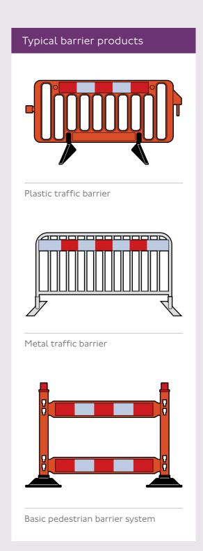
While the basic post and barrier system (see previous graphic) meets the minimum requirements, it may not always be suitable for all locations because of the large opening between barrier boards and posts. Barriers with smaller gaps and greater protection to mitigate the risk of unauthorised access (see figure to the right) should be considered, especially where high numbers of small children are expected.
